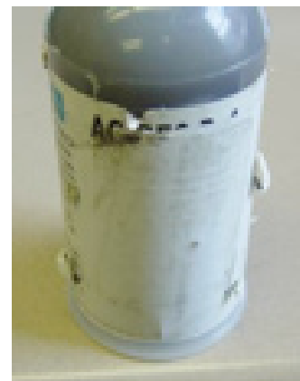
Figure 2: Scuffed Tag from Sealant Dispensing Gun
